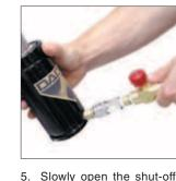
valve and allow gas spring to reach the desired charging pressure. After the gas spring has been charged to the desired pressure, CLOSETHE HOSE SHUT-OFF VALVE AND THE TANK SHUT-OFF VALVE.
