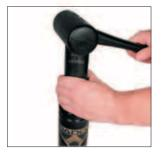
1. Stand the gas spring upright Make sure the rod is retracted in the tube. Place a Removal Sleeve (90.340.x) over the rod. Tap the sleeve until the Dust Cover (90.246.x) is loosened. Remove the Dust Cover and discard.
