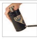
9S. Make sure the valve is in place and thread Port Plug (90.505.110) securely over top.
