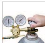
3. Open the main valve on the nitrogen tank.
