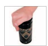
4. After all of the gas pressure is exhausted, be sure that the piston rod will freely extend and retract into the tube manually. If not, try depressing the valve again. If still unsuccessful, **STOP** and contact DADCO.
