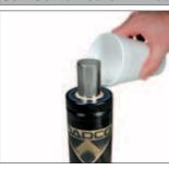
7. Check for leaks at the top of the tube around the rod and at the base around the valve compartment using vegetable oil or water.
