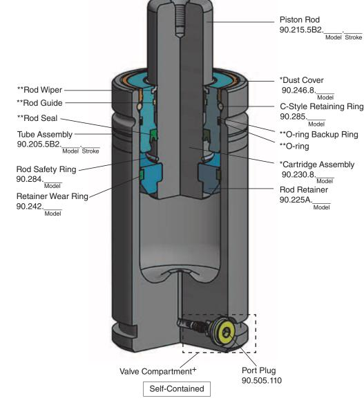
\*Included in the Repair Kit \*\*Included in the Cartridge Assembly
