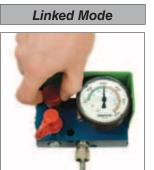
1L. To increase system pressure, set the regulator on the nitrogen tank to the desired level and fill the system through the control panel. To release pressure, open the drain valve on the control panel.
