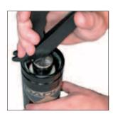
3. Remove the C-style Retaining Ring (90.285.x) using the C-Ring Removal Tool (90.355 or 90.356). Position the correct hooked end of the C-Ring Removal Tool below the c-ring. For best results lay cylinder horizontally and locate the tool near either end of the c-ring. See bulletin B15127A for more information.
