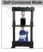
8S. Verify the pressure with a DADCO Load Cell using a Portable Test Stand (90.305.3) or an arbor press.
