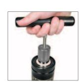
8. Thread T-Handle (90.320.x) into the end of the piston rod. Pull up on T-Handle until the top of the cartridge is past the c-ring. The rod must seat cartridge assembly fully (with the housing flush with end of cylinder). Make sure rod is extended to its proper stroke length. (Depress cartridge valve to facilitate full rod extension.)
