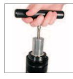
1. To remove the Cartridge Assembly, thread a T-Handle (90.320.x) into the rod end.
