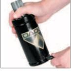
2S. To decrease gas spring pressure, depress the valve stem using a Valve Bleed Tool
