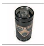
6. Position the top of the cartridge just below the retaining ring groove. The assembly cap is designed to locate the cartridge in this position.
