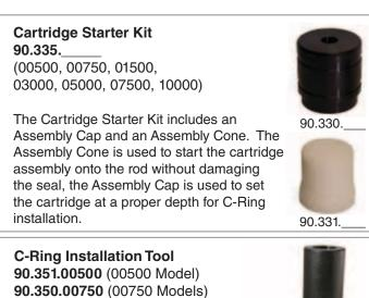
To insert the C-style retaining ring into the retaining ring
