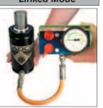
1L. Pipe all gas springs back to the control panel, making sure that all connections are tight and that gas spring rods are extended.
