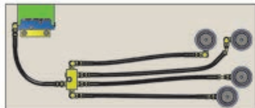
DADCO SMS® with (4) 90.10.03000 gas springs linked using 90.400 (Y-400) hose, fittings and a control panel.
