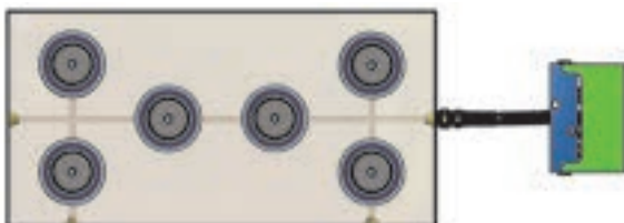
DADCO SMS-i® with (6) 90.10.05000 gas springs plumbed internally and connected to a control panel.
