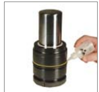
6. Extra oil should be applied to the housing o-ring, cushion seal and the inside of the housing.
