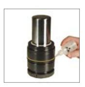
6. Extra oil should be applied to the housing o-ring, cushion seal and the inside of the housing.
