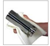
1. Slide the cartrige off the rod and lightly polish the rod surface with an emery cloth (600 grit). Inspect the finish of the rod for any scratches or gouges, if damaged it must be replaced.
