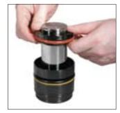
3. Tap or slide the cushion collar off from piston end. 90.10 Series Nitrogen Gas Springs will not have a cushion collar to remove.
