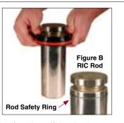
2. Install the new retainer halves and add the wear ring. Using a mallet or an Arbor Press, seat the collar against the rod retainers.
