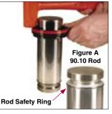
1a. Evaluate the position of the rod safety ring. If the ring is positioned like Figure A, lubricate the rod using some of the assembly oil and slowly tap the new cushion collar on the rod assembly from the top of the rod.
