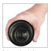
2. Inspect the tube for any damage, especially around the mouth. Polish out any scratches, if damage is severe the tube must be replaced. Wash, clean and dry the inside of the tube.
