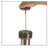
4. Fasten the cushion collar onto the rod retainer using the four collar retainer screws provided in the repair kit, torque value = 42 lb-in (5Nm).
