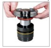
2. Remove the two retainer halves and discard.
