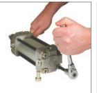
2. Remove the tie rod nuts from the rear head using a socket drive allen wrench. Retain nuts for use during reassembly.
