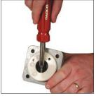
4. Remove the dampening washer, save for reassembly.
