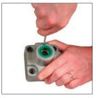
7. Use the notch in the head to remove the rod seal. Be careful not to damage or scratch the inside of the head. Discard the rod seal.
