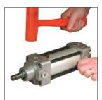
14. Replace the front head ensuring alignment of the ports between the front and rear heads, then insert the four tie rods. To ensure proper alignment, square the heads using a flat surface (ex., granite block).
