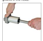
11. Remove the rod and piston assembly.
