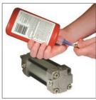
15. Replace the tie rod nuts using a medium strength liquid thread locker on the threads before re-installing. Alternate tightening of each tie rod nut a half turn until all tie rod nuts are secure. See page 2 for torque values. This completes the repair of your HP Series Air Cylinder.
