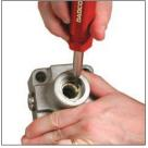
8. Remove the plastic bearings using a screwdriver to pop them out. Be careful not to damage or scratch the inside of the head.
