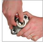
9. Replace the bearings by snapping them into the grooves.
