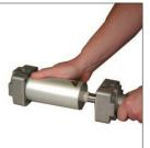
3. Remove the tie rods then remove the front head assembly.
