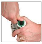
10. Install the new rod seal and set the front head aside for cylinder reassembly.
