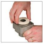
6. Insert the new front cushion seal with the flat side down. Reinstall the damping washer, be sure to line up the washer with the groove in the head.
