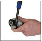
12. Remove and replace the piston seals, be careful not to scratch the surface of the piston. Guide tape will be loose and can be easily removed from the piston. Make sure the guide tape is in place before installation.
