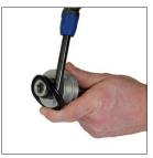
10. Remove the piston seals, being careful not to scratch the surface of the piston. Discard used seals. Guide tape will be loose when the piston is removed from the tube.
