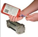
14. Replace the tie rod nuts using a medium strength liquid thread locker on the threads before re-installing. Alternate tightening of each tie rod nut a half turn until all tie rod nuts are secure, see page 2 for torque values. This completes the repair of your HP Series Air Cylinder.
