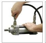
1. Unhook the cylinder from 2. Remove the tie rod the air supply.
