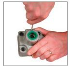
7. Use the notch in the head 8. Replace the rod seal with 9. Remove the rod and to remove the rod seal. Be careful not to damage or scratch the inside of the
