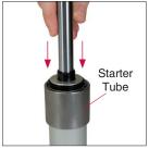
rod and piston assembly use DADCO's Starter Tube (refer to page 2). Place the starter tube on top of the tube and carefully guide the rod and piston assembly into the tube. Maintain alignment and ensure the piston seals and guide tape remain in place.
