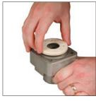
6. Insert the new front cushion seal with the flat side down. Reinstall the dampening washer, be sure to line up the washer with the groove in the head.
