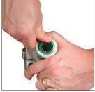
the new rod seal from the seal kit. Set the front head aside for reassembly of the cylinder.
