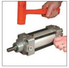
12. For installation of the 13. Replace the front head ensuring alignment of the ports between the front and rear heads, then insert the four tie rods. To ensure proper alignment, square the heads using a flat surface (ex., granite block).
