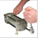
nuts from the rear head using a socket drive allen wrench. Retain nuts for use during reassembly.
