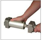
3. Remove the tie rods then remove the front head assembly.
