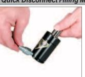
1. Thread the M6 end of the Quick Disconnect Filler Valve. (90.310.143), into the port of the gas spring. Connect the female end of the charging assembly to the charging nipple. The DADCO Pressure Analyzer. (90.315.5). can also be used for charging discharging and gauging pressure.
