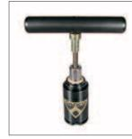
1. To remove the Rod and Cartridge Assembly thread a T-Handle, (90.320.1 or 90.320.2), into the rod end. Pull the entire assembly out of the tube. The spring body can be held in a vise (with soft jaws) while pulling out the assembly.
