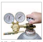
6. After all the springs in the system have been charged to the desired pressure, CLOSE THE HOSE SHUT-OFF VALVE AND TANK SHUT-OFF VALVE.
