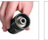
5. Place the rod and cartridge into the Tube Assembly. Depress the needle valve to release any back pressure. Position the top of the cartridge just below the retaining ring groove. The bore of the cartridge assembly is designed to stop the cartridge in this position. DO NOT force the cartridge down further into the tube.
