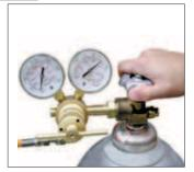
2. Open the main valve on the nitrogen tank.
