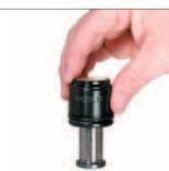
2. Position the new Cartridge Assembly over the rod, making sure that the wiper end marked "TOP" is facing up. While holding the cartridge vertically, slide the cartridge down the rod to the rod retainer
