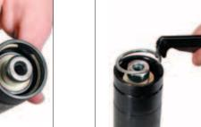
3. Remove the C-style Retaining Ring, (90.285.x.x), using a C-Ring Removal Tool, (90.355). Position the hooked end of the tool below the c-ring. For best results locate the tool near either end of the c-ring. (Use the Port Servicing Tool to pry out C-style Retaining Rings found in 13 mm stroke or shorter models.)
