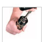
7. Thread the T-Handle, (90.320.1) or (90.320.2), into the end of the piston rod. Pull up on the T-Handle until the top of the cartridge is completely past the c-ring. The rod must seat the cartridge assembly fully before charging. The cartridge should be flush with the end of the cylinder. Make sure the rod is extended to its proper stroke length. (Depress the needle valve to facilitate full rod extension.)
