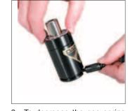
2. To decrease the gas spring pressure, depress the valve stem using a DADCO Valve Bleed Tool, (90.360.4).
