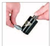
1. To increase the spring pressure, thread the Quick Disconnect Filler Valve, (90.310.143), into the port, set the regulator to the desired pressure and fill. The 90.315.5 may also be used to adjust pressure.
