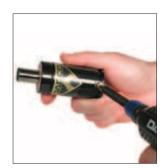
2. Remove the Port Plug, (90.607.110), located at the base of the spring. Retain parts for use during reassembly.
