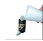
7. Check for leaks at the top of the tube around the rod and at the base around the valve compartment using mineral oil or water. Verify the pressure with a DADCO Load Cell using a DADCO Portable Test Stand, (90.305.3). NOTE: If spring is open-flow,
