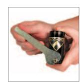
3. Unthread the service fitting and wipe with a clean cloth. Proceed to "II. Port Maintenance" Open Flow Mode, Step 1.
