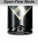
1. Check the port for deposits or burrs and clean thoroughly. Inspect the service fitting and replace if it shows signs of damage. Lubricate threads and seals on the fitting and thread the service fitting into the gas spring port.
