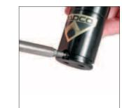
5B. Retrieve and replace the Valve Retaining Screw, (90.251). Proceed to step "III. C-Ring Removal."
