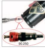
4B. Thread a new Needle Valve, (90.250), into the port until it fits snugly on the seat. Avoid over torquing the valve.
