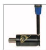
3. Keeping face and hands clear of the port, use the Valve Bleed Tool, (90.360.4), or Port Servicing Tool. (90.320.8). to depress the valve stem (90.250) or (90.260). Cover the port with a cloth to absorb discharge.
