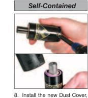
(90.246.x.x). Tap with a soft mallet until the top of the Dust Cover rests flush with the top of the Tube Assembly. The rod wiper should be visible. 9. Thread the Port Plug (90.607.110) into the port.
