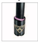
1. Stand the gas spring upright. Place a Removal Sleeve (90.340.x), longer than the stroke over the rod. Make sure to use the proper removal sleeve for the cylinder. Tap the sleeve until the Dust Cover, (90.246.x.x), is loosened. Remove the Dust Cover and discard.
