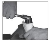
3. Lightly oil the body of the gas spring (Micro 90<sup>®</sup>/ Micro 180<sup>®</sup>) and install it into the Tube. Replace the rear head. Tighten using the Rear Head Removal Tool with a wrench or the Removal Kit to 180 lb-in / 20 N-m.
