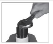
1. Wrap the SLN.090/SLN.180 cylinder body in a soft cloth. Clamp the cylinder face down in a vise so that the cylinder is secured. Remove the Rear Head using the Rear Head Removal Tool with a wrench or the Removal Kit.
