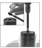
2. Oil the piping adapter, (90.270), then install into the bottom center port using an allen wrench. With a torque wrench, tighten the piping adapter to the appropriate torque value listed in the table.
