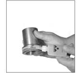
3. Once the new seal is pressed down evenly and positioned properly around the rod then snap the new piston rider around the rod. Lubricate the seal using the DADCO Assembly Oil and reinstall the rod assembly.
