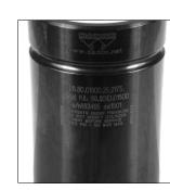
1. Choose the appropriate seal kit (98.801.D.x) by examining the laser mark on the tube for the seal kit number. If the laser mark does not have a D on the seal kit number, contact DADCO for repair. Note: Seal kits are not interchangeable among models.
