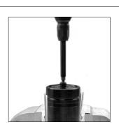
4. Remove the piping adapter, (90.270), located on the bottom of the spring with an allen wrench and retain for reassembly.
