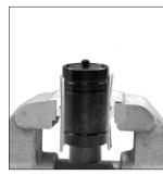
3. Position the gas spring upside down in a vise so that the cylinder is secured. Be sure to wrap the spring in cardboard to protect it from
