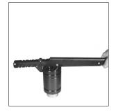
6 Insert the C-Style Retaining Ring, (98.285.80.x), in the retaining ring groove using a DADCO C-Ring Installation Tool, (90.352), or standard bench tools. Refer to bulletin B01101D for detailed instructions on how to use the C-Ring installation Tool.
