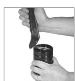
3. Once the hooked end of the tool is firmly seated below the c-ring, begin pushing it toward the outside of the gas spring can. The handles will close naturally, and the c-ring will be extracted as you complete this motion. Request the C-Ring Removal Tool Bulletin for more information.
