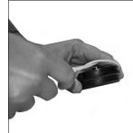
3. Using a small screwdriver, remove the O-Ring Backup, (98.249.80.x), and the O-Ring, (98.245.80.x), from the rear head, be careful not to scratch the inside of the groove. Discard both o-rings.
