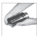
2. To decrease the gas spring pressure, depress the valve stem using a DADCO Valve Bleed Tool, (90.360.4), or a DADCO Pressure Analyzer, (90.315.5).
