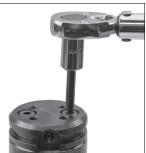
the screws to the appropriate torque value listed in the table.
