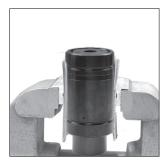
1. Position the gas spring upside down in a vise so that the cylinder is secured. Be sure to wrap the spring in cardboard to protect it from the vise.
