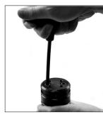
Remove the cap screws with washers from the bottom of the subplate and keep for reassembly.
