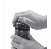
3. Align the subplate so that the piping adapter matches the hole in the subplate and the cap screw holes line up.
