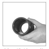
Inspect the tube assembly for any damage. Polish out any burrs at the bottom of the tube assembly to avoid damaging seals during the reassembly process. If there are any severe scratches in the finish contact DADCO for repair.
