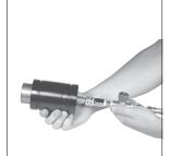
4. After the spring has been charged to the desired pressure, CLOSE THE HOSE SHUT-OFF VALVE AND TANK SHUT-OFF VALVE. Disconnect the charging assembly. The small amount of nitrogen trapped between the shut-off valve and filler valve will bleed off as you disconnect the fitting.
