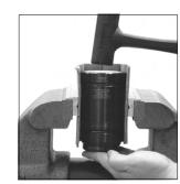
1. Wrap the cylinder in cardboard and place in a vise. With a soft rubber mallet, tap the rod down through the tube. This will push the rear head out at the same time. **Note:** You will need to guide the parts as they are pushed out. To avoid damaging the piston rod or bore do not let them drop onto a hard surface.
