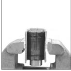
1. When exhausting pressure, position the gas spring upside down in a vise so that the cylinder is secured. Be sure to wrap the spring in cardboard to protect it from the vise.
