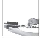
3. Slowly open the shut-off valve at the end of the charging hose and charge to a low pressure. Gradually increase the regulator setting to the desired pressure. Charging Pressure Range: 25-150 bar
