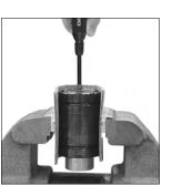
3. Keeping face and hands clear of the port, use the Valve Bleed Tool, (90.360.4), or the Port Servicing Tool, (90.320.8), to depress the Compact Valve (90.260). Cover the port with a cloth to absorb discharge.
