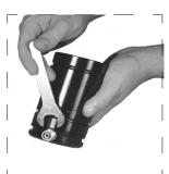
3. Remove the mount, if necessary, securing the cylinder to the plate. Unthread the service fitting and wipe with a clean cloth. Retain parts for use during reassembly.
