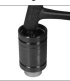
1. Hold the discharged gas spring upside down. Using a rubber mallet gently tap the rear head down into the tube. It may be necessary to depress the valve stem again to release any back pressure.
