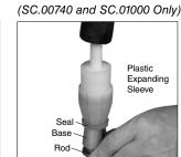
2A. It is necessary to use the Seal Installation Tool, (95.357D.00740 or 90.357D.01000 for the SC.00740 and SC.01000 models), to install the new seal. Place seal on base of tool and slide base over rod. Insert the plastic expanding sleeve over base. Using a soft rubber mallet tap the plastic sleeve until the seal is pushed down onto the rod.
