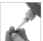
4. Apply serviceable thread locker to the bottom three threads of the cap screws with lock washers.
