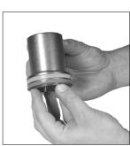
2B. Press the new seal down evenly until it is positioned properly around the rod.
