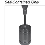
6. Make sure the Sealing Washer is in place and thread the Port Plug, (90.607.110 or 90.505.110), using the Port Servicing Tool, (90.320.8), securely over top.
