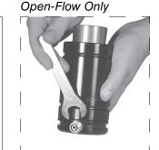
7. After testing all springs for leaks, the open-flow springs are ready to be re-linked in the system. If possible, once the springs are all linked back to the control panel, leave the system to sit fully charged overnight. If pressure has dropped indicating a leak verify that each connection is tight and test each fitting for a leak.
