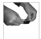
4. Place the rear head so the mounting holes are facing down. Install the O-Ring Backup, (98.249.80.x), and then the O-Ring, (98.245.80.x). The o-ring will be seated above the o-ring backup in the same groove. Verify that the o-ring backup and the o-ring do not twist when installing.
