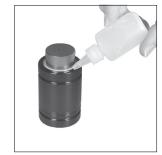
5. Check for leaks at the top of the tube around the rod and at the bottom around the valve compartment by using mineral oil. Do not use water. Verify the pressure with a DADCO Load Cell using a DADCO Portable Test Stand or an arbor press. NOTE: If spring is open-flow, the DADCO Pressure Analyzer, (90.315.5), must remain in place during testing.
