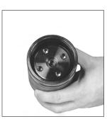
5. Reinstall the rear head into the tube. If necessary, depress the valve to release any back pressure.
