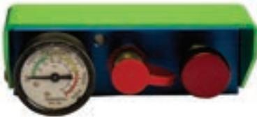
The DADCO Mini Convertible Control Panel is used to fill, drain and monitor the pressure of linked DADCO nitrogen gas springs from outside the die. The panel is compatible with SMS-i® and traditional linked systems and has five M6 ports, a high pressure gauge, a quick disconnect fill valve, a bleed valve and a rupture disk to prevent over pressurization. To allow for maximum versatility when linking, the panel is available with a variety of fitting connections.
