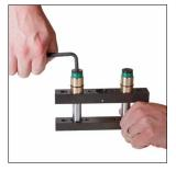
1B. Install the Upper Mount with Bronze Bearings onto the Guide Rails. Add 2-3 drops of serviceable threadlocker to each Rod Retaining Screw. Install the two screws with Dampening Devices using an 8 mm allen wrench to **600 lb.-in** / **67 N-m**.
