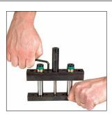
4. Install the two Mount Screws using a 5 mm allen wrench to **175 lb.-in** / **20 N-m**.
