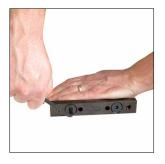
4A. Add 2-3 drops of serviceable threadlocker to the Plate Screws and install them into the Rail Plate using an 8 mm allen wrench to 600 lb.-in / 67 N-m.
