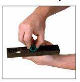
1A. Inspect the Plate Wiper located in the Upper Mount for wear. If the Plate Wiper, (*SR463378, sold separately*), is damaged it must be replaced.
