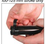
2. Remove the two halves of the Piston, (SA257770). Clean and inspect. If the Piston is damaged it must be replaced. Note the proper orientation of the piston halves for reassembly.
