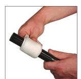
1. Clean the Guide Rod surface and inspect for deformation in the retaining groove area. If the Guide Rod is damaged it must be replaced.
