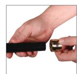
3. Slide the Bearing, (SA407770), off the Guide Rod and discard. Retain the rod for inspection and reuse.
