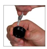
8. Add 2-3 drops of serviceable threadlocker to the threads of the rear head. Replace the Rear Head. Tighten using the Rear Head Removal Tool Kit, (SLN.HR.090), and a wrench to 180 lb,-in / 20 N⋅m.
