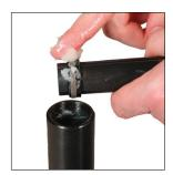
5. Lightly coat the inside of the Tube Assembly and Piston Rider with the DADCO assembly grease included in the repair kit.
