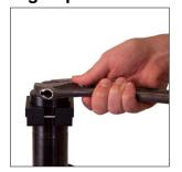
1. Wrap the SLN.090 cylinder body in a soft cloth. Clamp the SLN.090 face down in a vise so that the cylinder is secured. Remove the Rear Head, (SA107770), using the Rear Head Removal Tool Kit, (SLN.HR.090), and a wrench.
