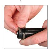
4. Snap the new Piston Rider, (SA411661), onto the Piston. Be careful not to deform the Piston Rider.
