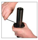
1. Remove the two screws from the bottom of the mount using a 2.5 mm allen wrench.
