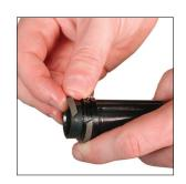
1. Remove the Piston Rider, (SA411661), from the Piston and discard. If repairing a 25-80 mm stroke cylinder, proceed to "V. Cleaning & Inspection," step 1.
