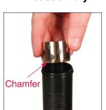
1. Install the Bearing, (SA407770), into the Tube. Make sure the Bearing is positioned correctly, with the chamfered side facing the Tube Assembly.
