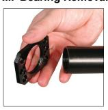
1. Slide the Lower Mount, (SA557771), off the Tube of the Tube Assembly. Assembly.
