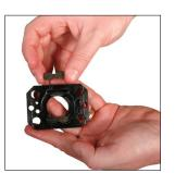
3. Remove the two Rod Keys, (SA857770), from the Upper Mount, (SA557770), and inspect for wear. If the keys show signs of wear on only one side they may be turned 180 degrees and reused. If they show signs of wear on both sides, they must be replaced.
