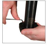
2. Install the Lower Mount, (SA557771), and Upper Mount, (SA557770), with Rod Keys onto the Tube Assembly. Install the two mount screws into the Lower Mount with a 2.5 mm allen wrench to 36 lb-in / 4 N-m. If repairing a 25-80 mm stroke cylinder, proceed to step 4.
