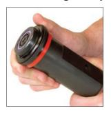
3A. Inspect the Piston and Cushion for damage or wear. If the Piston or Cushion is damaged it must be replaced. SLN.300 Lifters manufactured after week 18 of 2007 (md1807) will have a new Piston, Piston Rider and Cushion. NOTE: The Piston. Piston Rider and Cushion retrofit lifters manufactured before week 18 of 2007 (md1807).
