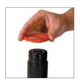
3. Slide the Cushion off the Guide Rod. NOTE: If Cushion shows signs of damage it must be replaced.
