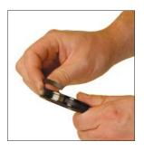
4. Remove the Rider from the Piston and inspect. Clean the Piston. Snap the new Rider onto the Piston, set aside for reassembly. Return to DADCO's SLN.300 Maintenance Bulletin VII. Internal Rod Removal.
