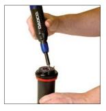
1. Remove the Retaining Ring from the Piston using the Port Servicing Tool's small flat bit.
