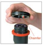
5B. Install the Piston onto the Guide Rod with Piston chamfer facing toward the cartridge.
