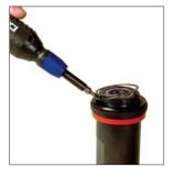
6. Install the new Retaining Ring by pressing into place with the Port Servicing Tool's small flat bit. The Retaining Ring must be completely seated in the square groove. Return to DADCO's SLN.300 Maintenance Bulletin VIII. Seal Kit Replacement and Reassembly, step 7.
