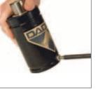
9. Install the new Dust Cover, (90.246.U.x). Tap with a soft mallet until the top of the Dust
