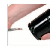
3S. Thread a new Compact Valve, (90.260), or Cartridge Valve (90.265), into the port until it fits snugly on the seat. Avoid over torquing the valve.
