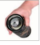
2. Reposition the DADCO Removal Sleeve and only continue tapping until the rod cartridge assembly is slightly below the retaining ring
