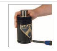
2S. Remove the Compact Valve, (90.260), or Cartridge Valve, (90.265), by unscrewing it with the Port Servicing Tool, proceed to step 2S, otherwise (90.320.8). leave the valve undisturbed and proceed to "III. C-Ring
