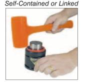
9. Install the new Dust Cover, (90.246.U.x). Tap with a soft mallet until the top of the Dust Cover rests flush with the top of the can. The rod wiper should be visible.
