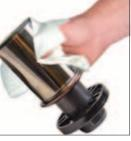
3. Inspect the Tube Assembly for any damage, especially around the mouth of the Tube Assembly. Lightly polish out any scratches at the mouth of the Tube Assembly to avoid damaging seals during the reassembly process. If damage to the Tube Assembly is severe it must be replaced Wash, clean and dry the inside thoroughly.
