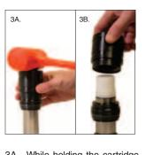
3A. While holding the cartridge vertically tap the Assembly Cap to drive the cartridge down the rod. Be careful not to force the over the Assembly Cone, cartridge at an angle as the seal could become damaged.
