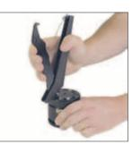
Remove the C-style Retaining Ring, (90.285.x.), using a C-Ring Removal Tool, (90.356 or 90.355). Position the hooked end of the tool below the c-ring. For best results locate the tool near either end of the c-ring.
