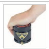
Verify that all pressure is relieved by manually retracting the piston rod into the tube. If the rod will not fully retract release the remaining pressure. If still unsuccessful stop and contact DADCO.
