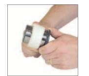
1. Lightly polish the rod surface 2. Inspect the Tube Assembly with an emery cloth (600 grit). for any damage, especially Inspect the finish of the rod for around the mouth of the Tube any scratches or gouges. If the Assembly. Lightly polish out rod is damaged it must be any scratches at the mouth replaced. of the Tube Assembly to avoid damaging seals during the reassembly process. If damage to the Tube Assembly
