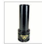
Stand the gas spring upright. Place a removal sleeve, (90.340.x), longer than the stroke over the rod. Tap the sleeve until the Dust Cover. (90.246.U.x), is loosened. Remove the Dust Cover and
