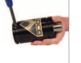
4S. After all of the gas pressure is exhausted, be sure that the piston rod will freely retract into the tube manually. If not, try depressing the valve again. It still unsuccessful stop and contact DADCO.
