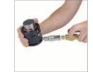
After the spring has been charged to the desired pressure, CLOSE THE HOSE SHUT-OFF VALVE AND TANK SHUT-OFF VALVE. Disconnect the charging assembly from the charging nipple. The small amount of nitrogen trapped between the shut-off valve and used to verify pressure and
