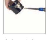
Valve, (90.260), or Cartridge Valve, (90.265), by unscrewing is leaking pressure or sticking it with the Port Servicing Tool, (90.320.8).
