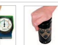
2L. Verify that all pressure is relieved by manually retracting the piston rod into the tube. If the rod will not fully retract release the remaining pressure. If still unsuccessful stop and contact DADCO.
