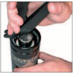
3. Remove the C-style Retaining Ring, (90.285.x.), using a C-Ring Removal Tool, (90.356 or 90.355). Position the hooked end of the tool below the c-ring. For best results locate the tool near either end of the c-ring.
