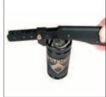
6. Insert the C-Style Retaining Ring in the retaining ring groove using a DADCO C-Ring Installation Tool, (90.351.00500 or 90.352). Be sure the C-Style Retaining Ring is fully seated in the retaining ring groove.
