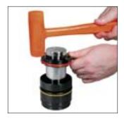
1. Tap a new cushion collar onto the rod assembly from the groove end.
