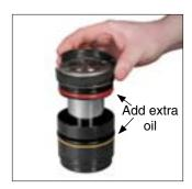
4. Add the wear ring. Extra oil should be applied to the housing o-ring, seal and the inside of the housing.
