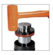
2. Using the mallet or an Arbor Press, seat the collar against the rod safety ring squarely. If retainer won't install, STOP and contact DADCO.
