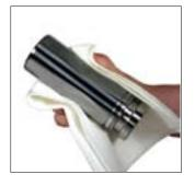
2. Lightly polish the rod surface with an emery cloth (600 grit). Inspect the finish of the rod for any scratches or gouges. If the rod is damaged it must be replaced.
