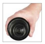
3. Inspect the Tube Assembly for any damage, especially around the mouth. Polish out any scratches at the mouth to avoid damaging seals during the reassembly process. If damage is severe it must be replaced. Wash, clean and dry the inside of the Tube Assembly. Be sure to clean the retainer halves.
