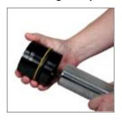
1. Slide the cartridge off the rod and discard.
