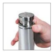
4. Place the new Rod Safety Ring on from the rear end of the rod. Position the new cartridge assembly over the rod with the wiper end marked "TOP" facing up. Slide the cartridge down the rod.
