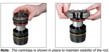
5. Remove two retainer halves.
