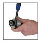
13. Remove the piston seals, being careful not to scratch the surface of the piston. Discard used seals. Guide tape will be loose when the piston is removed from the tube.
