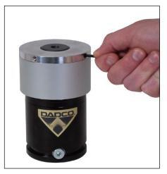
3. Tighten both screws using a 3 mm allen wrench.
