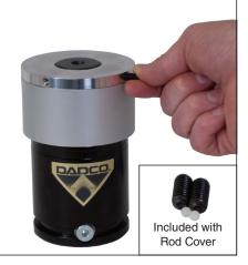
Install the two nylon locking balls and cup point set screws into the two holes in the rod cover. Nylon locking balls and retaining screws are included with the rod cover.
