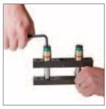
1. Remove the two Rod Retaining Screws, (with Dampening Devices), from the bottom of the lifter using an allen wrench. If necessary, wrap the SL2 in a soft cloth and clamp it in a vise.
