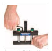
4. Install the Mount Screws using an allen wrench to the appropriate torque specification.
