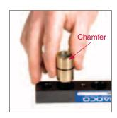
5. Install the new Bearings with Snap Rings, into the Upper Mount.
