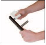
1. Clean the Guide Rails attached to the Rail Plate, and inspect the surface for deformation. If the Guide Rails are damaged they must be replaced, proceed to Step 2. If the Guide Rails do not need to be replaced proceed to "IV. Reassembly" step 1.
