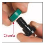
3. Install the new Dampening Devices onto the screws with the chamfer side facing the screw head.
