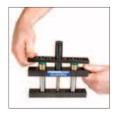
2. Pull the mount apart and slide the Lower Mount off the Gas Spring, (C.090.\_\_.BK, C.180.\_\_.BK or L.300.\_\_). The L.300 gas spring may be repaired or replaced; refer to maintenance bulletin #B01103F for more information.
