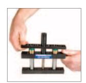
5. Install the Lower Mount over the Gas Spring.
