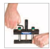
6. Install the Mount Screws using an allen wrench to the appropriate torque specification.
