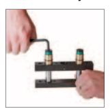
1. Install the Upper Mount with Bearings onto the Guide Rails. Add 2-3 drops of serviceable threadlocker to each rod retainer screw before installing. Tighten the two Rod Retaining Screws (with Dampening Devices) using an allen wrench to the appropriate
