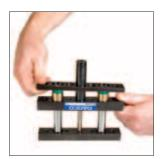
3. Install the Lower Mount over the Gas Spring.
