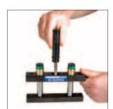
3. Slide the Gas Spring out of the Upper Mount. If replacing or repairing the Gas Spring only, proceed to step 4. To continue maintenance of the SL2 with replacement parts from the repair kit, proceed to "II. Bearing Replacement" step 1.
