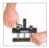
1. Remove the Mount Screws from the bottom of the lifter using an allen wrench.
