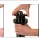
2. Place Removal Sleeve (90.340.00750 for SLC.500. 90.341.00800 for SLC.800) over rod. Tap sleeve until Dust Cover (90.246.x) is loosened. Remove Dust Cover and discard.
