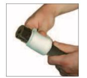
1. Clean the Guide Rod surface and inspect for deformation in the retaining groove area. If the Guide Rod is damaged it must be replaced.
