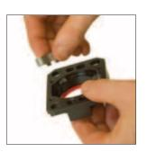
3. Remove the two Rod Keys (SQ853340) from the Upper Mount (SQ553335) and inspect for wear. If they show signs of wear, they must be replaced.
