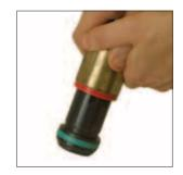
2. Use Bearing to install the Cushion Ring. The Cushion Ring should seat on top of Piston Retainer. Slide bearing off guide rod when complete.
