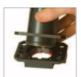
4. Install new Rod Wiper followed by the Rod Keys. Line up Rod Keys before torquing mount into place. Install and tighten Upper and Lower mounts. Install the two mount screws into the Lower Mount with a 3.0 mm allen wrench to 60 lb<sub>f</sub>-in / 6.8 N·m.
