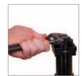
3. To verify **Micro 180**° gas spring force before installation, refer to the Micro Load Cell Bulletin, B07108. Lightly oil the body of the **Micro 180**° gas spring and install it into the Tube. Add 2-3 drops of serviceable threadlocker to the threads of the rear head. Replace the rear head. Tighten using the Rear Head Removal Kit (SLN.HR.180) to **180 lb**<sub>f</sub>-in / **20 N·m**.
