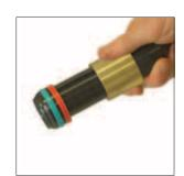
2. Slide the Bearing (SQ403335) off Guide Rod and discard. Retain the rod for inspection and reuse. NOTE: Bearing appearance may differ slightly.
