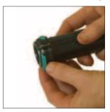
1. Snap the new Piston Rider (BQ419335) onto the Piston. Be careful not to deform the Piston Rider.
