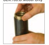
3. Install the Bearing (SQ403335) into the Body Tube.
