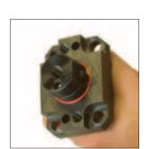
6. Place the Guide Rod into the Body Tube. Make sure the Guide Rod is properly aligned to the Rod Keys.
