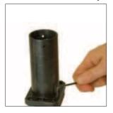
1. Remove the two screws from the bottom of the mount using a 3.0 mm allen wrench.
