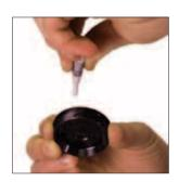
8. Add 2-3 drops of serviceable threadlocker to the threads of the rear head. Replace the rear head. Tighten using the Rear Head Removal Kit (SLN.HR.180) to 180 lb<sub>e</sub>-in/20 N·m.
