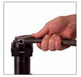
1. Clamp the SLN.180 face down in a vise so the cylinder is secured. Remove the Rear Head (SQ103335) using the Rear Head Removal Kit (SLN.HR.180) and a wrench.
