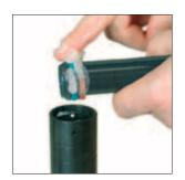
5. Lightly coat the inside of the Body Tube, Piston Rider and Cushion Ring with the DADCO assembly grease included in the repair kit.
