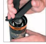
3. Remove the C-style Retaining Ring (90.285.x)using the C-Ring Removal Tool (90.356 or 90.355). Position the correct hooked end of the C-Ring Removal Tool below the c-ring. For best results locate the tool near either end of the c-ring.
