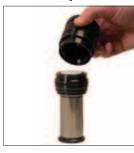
2. Thread Assembly Cone (90.331.x) from Cartridge Starter Kit (90.335.x) onto rod. Slide Cartridge Assembly over the Assembly Cone, making sure that the wiper end marked "TOP" is facing up. Place Cartridge Assembly Cap (90.330.x) from Cartridge Starter Kit on top of Cartridge Assembly.
