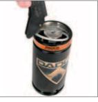
4. Once the hooked end of the tool is firmly seated below the c-ring, begin pushing it toward the outside of the gas spring can. The handles will close naturally, and the c-ring will be extracted as you complete this motion.
