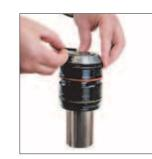
7. Snap Retainer Wear Ring around Rod Retainer. Apply oil from bottle of assembly oil to coat the cushion collar seal and cartridge o-ring.
