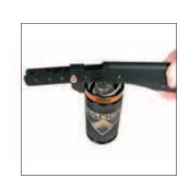
11. Insert the C-Style Retaining Ring (90.285.x) in the retaining ring groove using a DADCO C-Ring Installation Tool (90.352) or standard bench tools. Be sure C-Style Retaining Ring is fully seated in retaining ring groove.
