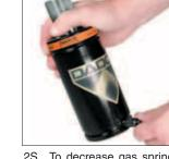
pressure, depress the valve stem using a Valve Bleed Tool (90.360.4) and release pressure in a controlled
