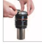
3. Remove the Retainer Wear Ring (90.242.x)from the Rod Retainer (90.225A.x).
