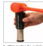
While holding the cartridge. vertically tap the Assembly Cap (90.330.x) to drive the cartridge down the rod. Be careful not to force the cartridge at an angle as the seal could become damaged.
