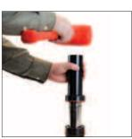
5. Using the Removal Sleeve (90.340.x) tap new Cushion Collar Assembly, making sure that the end marked "TOP" is facing up, onto rod from piston end using a soft rubber mallet or arbor press. Seat collar against rod safety ring squarely.
