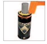
10. Install the new Dust Cover. Tap with a soft mallet until the top of the Dust Cover rests flush with the top of the can. The rod wiper should be visible. Thread Port Plug into secondary exhaust port .
