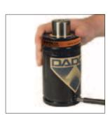
3. Replace the damaged valve. Use the Port Servicing Tool (90.320.8) to thread the new valve (90.265 or 90.260) into the port until it fits snugly on the seat. Avoid over torquing the valve
