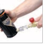
and allow gas spring to reach the desired charging pressure. After the gas spring has been charged to the desired pressure, CLOSETHE HOSE SHUT-OFF VALVE AND THE TANK SHUT-OFF VALVE.
