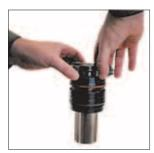
4. Remove the two halves of the Rod Retainer. Clean Rod Retainer and Retainer Wear Ring, set aside for reassembly.
