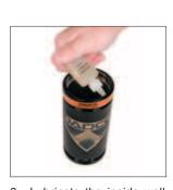
8. Lubricate the inside wall of the tube with remaining contents of the bottle of assembly oil.
