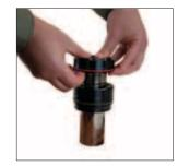
5. Tap or slide Cushion Collar Assembly (90.235.x) off rod from piston end and discard
