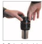
6. Replace the two halves of the Rod Retainer behind Cushion Collar Assembly. If retainer will not install, STOP and contact DADCO.
