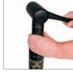
1. Stand the gas spring upright. Make sure the rod is retracted in the tube. Place a Removal Sleeve (90.340.x) over the rod. Tap the sleeve until the Dust Cover is loosened. Remove the Dust Cover and discard.
