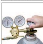
3. Open the main valve on the nitrogen tank.
