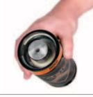
2. Reposition the Removal Sleeve and continue tapping until the rod cartridge assembly is slightly below the Retaining Ring groove. DO NOT force the cartridge down further into the Tube Assembly.
