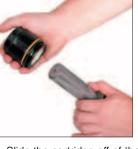
6. Slide the cartridge off of the rod and discard. Retain rod for inspection and possible reuse.
