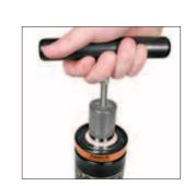
12. Thread T-Handle (90.320.2) into the end of the piston rod. Pull up on T-Handle until the top of the cartridge is past the c-ring. The rod must seat cartridge assembly fully (with the housing flush with end of the tube assembly). Make sure rod is extended to its proper stroke length. (Depress valve and secondary exhaust port to facilitate full rod extension).
