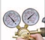
1S. To increase spring pressure, thread the Quick Disconnect Charging Nipple (90.310.111) into the port, set the regulator to the desired pressure and fill. DADCO's Pressure Analyzer (90.315.5) may also be used to adjust pressure.
