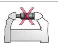
Do not compress gas springs in an unsafe manner. Never compress in a vice or clamp outside a die; damage can result. Never strike the rod with a hammer to test for pressure.
