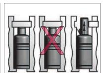
Sudden release will cause gas spring to exhaust. Restricting rod travel will help prevent gas spring damage.
