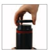
2. Remove the guide rod retaining key by sliding it off the Guide Rod. Retain the key for reassembly
