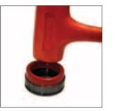
7. Install the new dampener into the Rod Retainer. Using a soft rubber mallet make sure the dampener retaining lip is completely seated into the retainer
