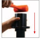
1. Using a soft rubber mallet install the Guide Retainer onto the Guide Rod
