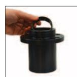
3. Remove the two middle bushings from the guide retainer. Discard used bushings. Inspect the Guide Retainer for any damage. Wash and dry the inside thoroughly.
