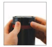
3. Remove the two halves of 4. Remove the dampener the rod retainer from the Guide backing ring and then the Rod and retain for reassembly. dampener from the Guide Rod. Retain the ring for reassembly
