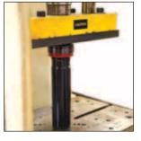
Dampener Assembly evenly onto the Guide Rod using a hydraulic press or a mediumsized arbor press. The assembly will snap into
