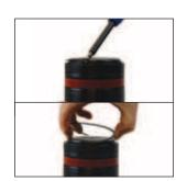
1. Remove the rod retainer ring located at the bottom of the guide rod using a screwdriver. Retain ring for reassembly
