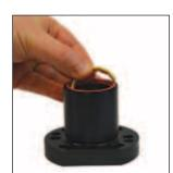
9. Install the third new bushing into the bottom of Guide Retainer. To insert, Overlap the gap portion and push the bushing into place past the excluder/dampener. Once all the bushings are installed, use all the grease supplied in the kit to grease the bushings.
