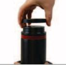
4. Install the rod retainer key over the rod retainer.
