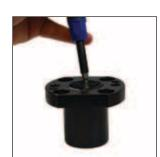
5. Remove the rod wiper using a small screwdriver and discard. Then remove the middle busing. Inspect the Guide Retainer for any damage. Wash and dry the inside thoroughly.
