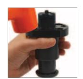
10. Install the Guide Rod into the Guide Retainer using a soft rubber mallet.
