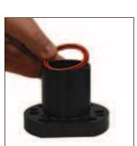
8. Install the new excluder/dampener into the bottom of Guide Retainer. Check to see it is well seated.
