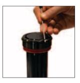
12. Install the safety wire ring onto the Rod Retainer by hand using a small screw driver to make sure it properly seats into the groove.
