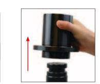
5. Pull the Guide Retainer off the Guide Rod. You may need to use a soft rubber mallet. A vise, with soft jaws, may be used to secure the Guide Rod if needed.
