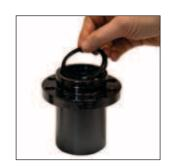
5. Install a new wiper into the top of Guide Retainer. Check to see it is well seated.
