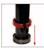
6. Remove the Rod Retainer from the Guide Rod. If needed, a vise with soft jaws may be used to secure the Guide Rod. Wash, clean and dry the Guide Rod thoroughly.
