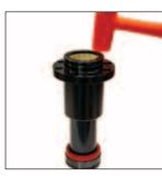
1. Install the Guide Rod into the Guide Retainer using a soft rubber mallet
