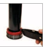
5. Using a utility knife, cut the dampener to remove it from the Guide Rod, and discard
