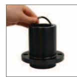
4. Install the bottom wiper (if it was present in step 1), then install the bottom bushings by overlapping the gap portion and placing it into the Guide Retainer
