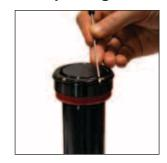
1. Remove the safety wire 2. Remove the three set screws ring from the outside of the Rod Retainer using a small screwdriver. Retain the ring for reassembly.
