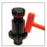
Remove the Guide Rod from the Guide Retainer using a soft rubber mallet. A vise, with soft jaws, may be used to secure the Guide Retainer if needed.
