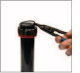
9. Install the rod retainer wire ring onto the Guide Rod using a set of external snap ring pliers.
