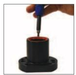
3. Remove the excluder/ dampener from the Guide Retainer and discard.
