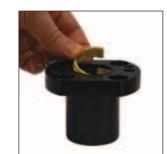
4. Remove the top bushing from he Guide Retainer using a small screwdriver and discard.
