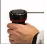
11. Install the three set screws into the Rod Retainer with Dampener Assembly using a 3 mm allen wrench.
