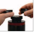
3. Install the two halves of the rod retainer.
