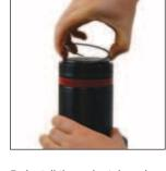
5. Install the rod retainer ring.
