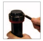
4. Remove the rod retainer wire ring using a small screwdriver or external snap ring spreaders. If needed, a vise, with soft jaws. may be used to secure the Guide Rod. Retain the ring for reassembly.
