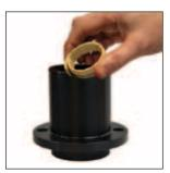
4. Install the two new middle bushings one at a time by overlapping the gap portion and placing them into the Guide Retainer.
