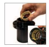
6. Install the top bushing by overlapping the gap portion and placing it below the wiper into the Guide Retainer. The bushings may not seat properly if the wiper is not seated properly.
