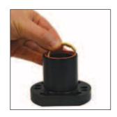
2. Remove the bottom bushing from the Guide Retainer using a small screwdriver and discard.
