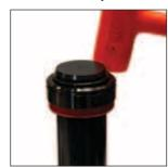
3. Tap down the Rod Retainer on the Guide Rod using a soft rubber mallet.
