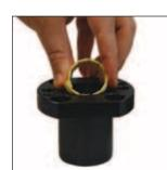
7. Install two new bushings, one at a time, into the top of the Guide Retainer. To insert, Overlap the gap portion and push them into place.
