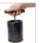
9. Thread the T-Handle, (90.320.1 or 90.320.2), into the end of the piston rod. Pull up on the T-Handle until the top of the cartridge is completely past the c-ring.
