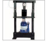
2S. Check for leaks at the top of the tube around the rod and at the base around the valve compartment by using mineral oil or water to test for leaks. Verify the pressure with a DADCO Load Cell using a DADCO Portable Test Stand, (90.305.3).
