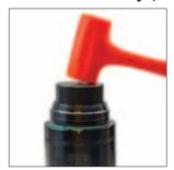
7. Place the rod and cartridge into the Tube Assembly. Use the Valve Bleed Tool, (90.360.4), or Port Servicing Tool, (90.320.8), to depress the valve to release any back pressure. Position the top of the cartridge just below the retaining ring groove.
