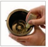
6. Lubricate the inside wall of the Tube Assembly with all remaining DADCO Assembly Oil
