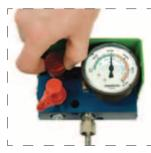
2L. Attach Charging Assembly (90.310.040) to the quick disconnect filler valve on the control panel and pressurize the system. Do not exceed the maximum charging pressure of 150 bar (2175 psi).
