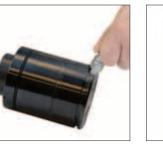
1S. Thread the Quick Disconnect Charging Nipple, (90.310.111), into the port of the gas spring. Connect the female end of the charging assembly to the charging nipple and pressurize the gas spring. Do not exceed the maximum charging pressure of 150 bar (2175 *psi*). The DADCO Pressure Analyzer, (90.315.5), can also be used for charging, discharging and gauging pressure in selfcontained gas springs.
