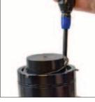
10. Insert the Spirolox Retaining Ring in the retaining ring groove using the Port Servicing Tool, (90.320.8). Be sure the Spirolox Retaining Ring is fully seated in the groove.
