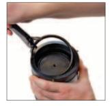
5. Once the hooked end of the tool is firmly seated below the c-ring, begin pushing it toward the outside of the gas spring can. The handles will close naturally, and the c-ring will be extracted as you complete this motion. For a detailed explanation of c-ring removal see bulletin B15127A.
