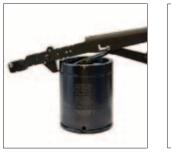
8. Insert the C-Style Retaining Ring in the retaining ring groove using a DADCO C-Ring Installation Tool, (90.352). Be sure the C-Style Retaining Ring is fully seated in the retaining ring groove. For a detailed explanation of c-ring installation, see bulletin B01101D.
