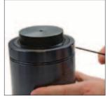
11. Using a 2 mm allen wrench, tighten the three set screws at the top of the gas spring.
