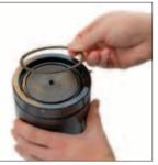
2. Continue moving around the Spirolox Retainer Ring until removed. Keep the ring for reassembly.
