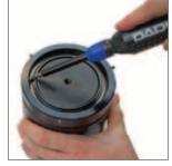
1. Using the Port Servicing Tool, (90.320.8), start at the tab and begin to pry up the Spirolox Retainer Ring.
