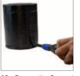
2S. Remove the Compact Valve, (90.260), by unscrewing it with the Port Servicing Tool, (90.320.8). Thread a new Compact Valve, (90.260), into the port until it fits snugly on the seat. Avoid over torquing the valve.
