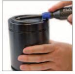
2. Using the Port Servicing Tool, (90.320.8), pry the Wiper Retainer from the top of the gas spring and retain for reassembly.
